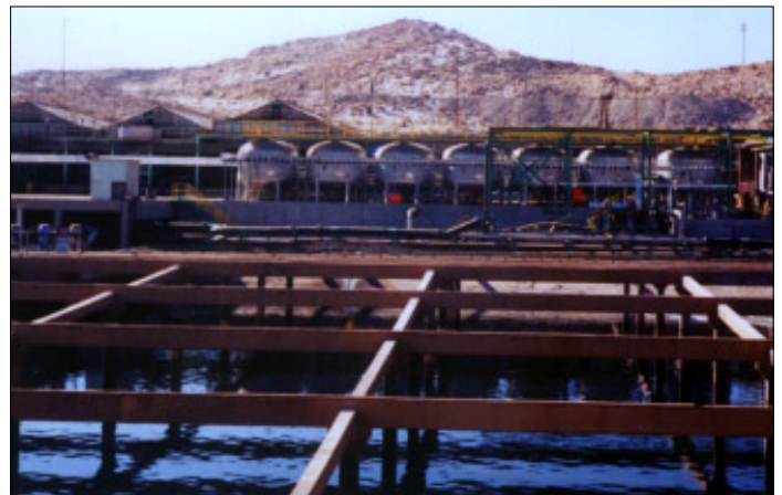
The Andes Mountains surround the seven S&L DI-SEP® SX Electrolyte Filters at the Cerro Verde Copper Mine (top) located near Arequipa, Peru. These filters remove virtually all impurities allowing for the production of 99.99% pure copper plate.
